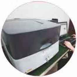
Energy dispersive X-ray fluorescence spectrometer To detect the harmful materials, according with the demand of EU standard
