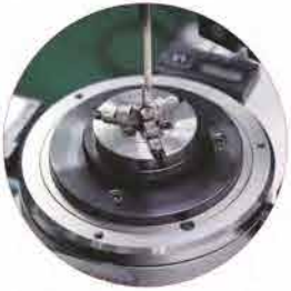
Roundness measuring instrument imported from Japan, high degree of accuracy(0.01um)
